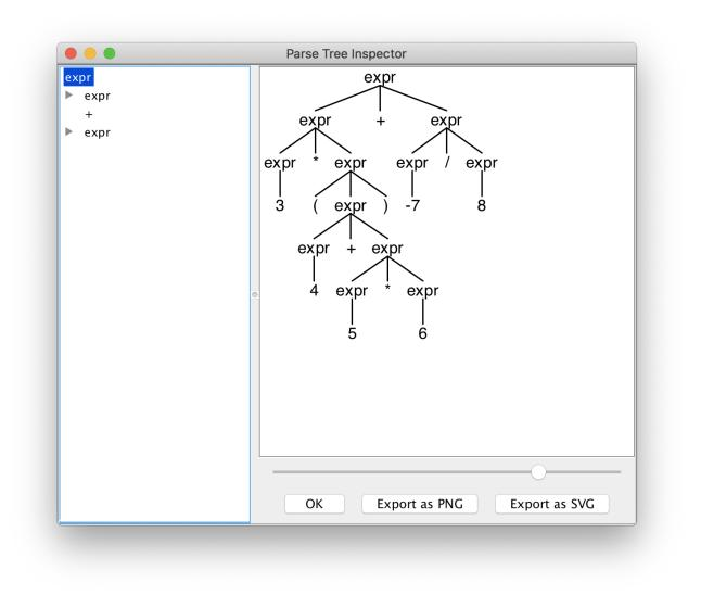
Figure 1: The resulting derivation tree when parsing the expression 3 \* (4 + 5 \* 6) + -7 / 8 using the SimpleArith grammar.
